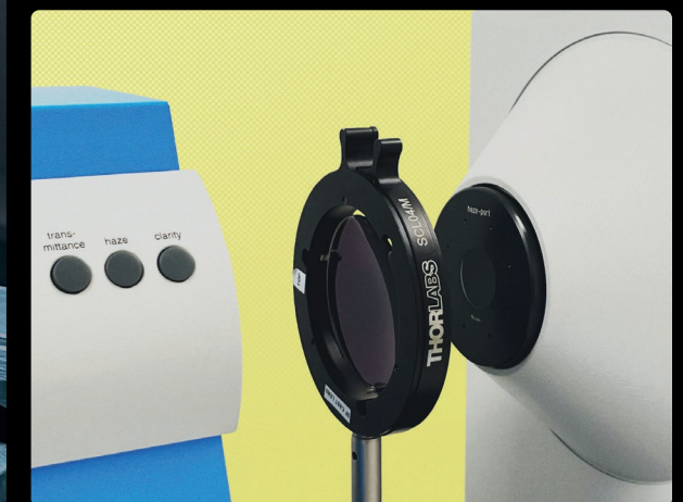
BOTTOM RIGHT: OPTICAL LENS TESTING; TRANSMISSION / HAZE / SPECTRO
